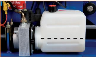
The correct level in this condition is approximately 1/3 from the base of the tank, as indicated by the line.
