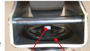
Castor mounting bolt Swivel bearing head should feel free to rotate and not loose
