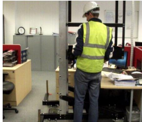
7. **▲ DANGER** Check rung-locks are fully engaged. If locks are not engaged repeat steps 5 to 14.
