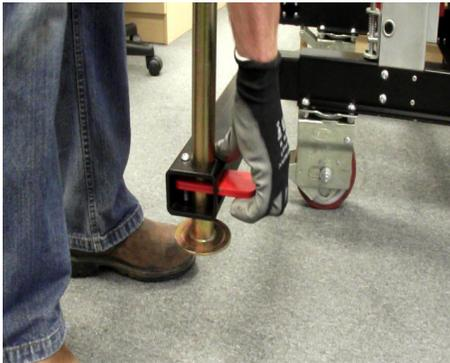
5. Check that the rung-lock bungee cord on ladders is loose by pulling the top end of the cable straight up and releasing.
