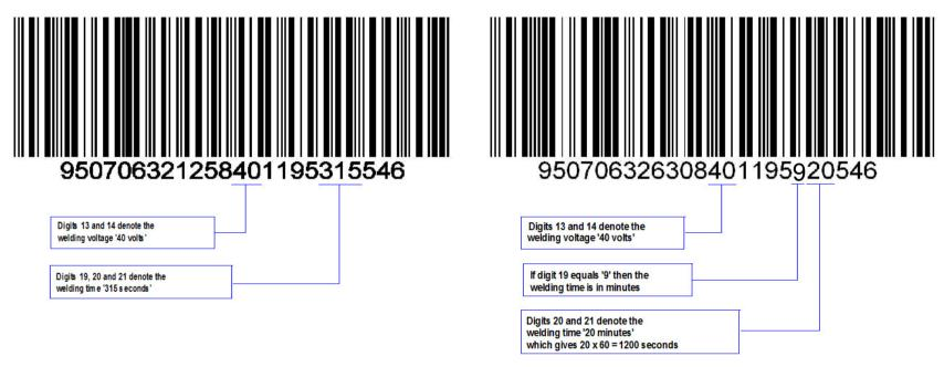
Figure 1 above shows the welding voltage required is 40 volts and that the welding time is 315 seconds.
